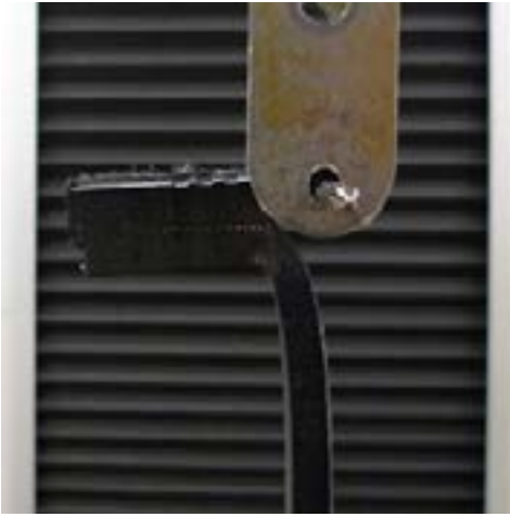
Figure 1. Peel test setup as per ISO 13954
