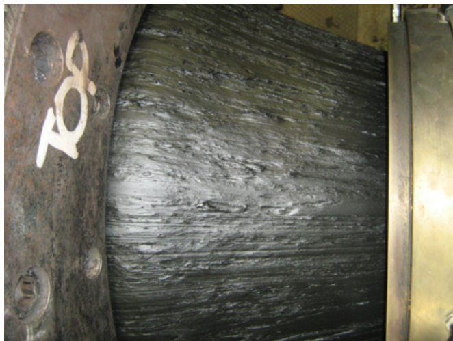
Figure 2. Excessive moisture in the pipe compound affects the quality of the finished pipe, including the appearance of the outer surface of the pipe wall. Picture shows moisture affected pipe surface during pipe manufacturing between the extruder die and sizing calibrator.
