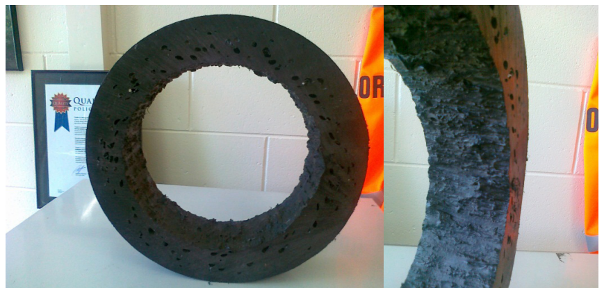
Figure 1. Effects of excessive moisture in pipe compound on PE pipe: voids in the pipe wall (left) and rough surface of inner pipe wall (right).
