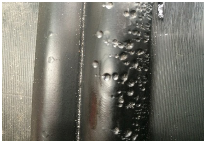
Figure 3. Example of a butt weld of black PE pipe affected by moisture at the jointing surface.
